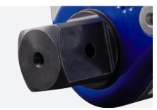
The MXT pioneered this new system for more powerful breakout and faster tightening. The secondary pawl inside the tool prevents the ratchet from turning opposite of the direction it is being driven.
